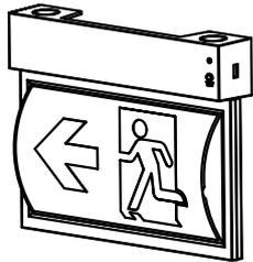
Remove the pictogram on the unit, select other pictogram you need then insert into slot of panel.
