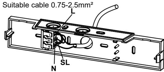
Connect the AC supply wire to terminal block. Refer to wiring instruction shown below.
