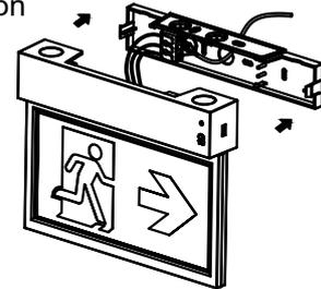
Snap AC supply on PCBA and then snap fixture to mounting plate.
