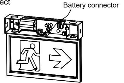
Connect battery male and female connector inside of mounting bracket.
